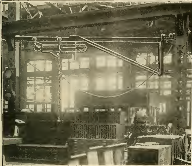
CRANE AND HOIST FOR DRIVING BOXES, IN THE DRIVING BOX SECTION OF THE LOCOMOTIVE SHOP. (See page 364.)
